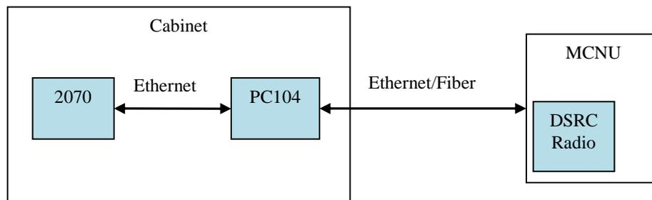
**Figure 5.3** SPaT Components as Implemented at PATH Intelligent Intersection
