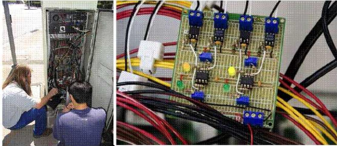
**Figure 5.1** Analog signal current “sniffer” as installed at a VII California intersection
